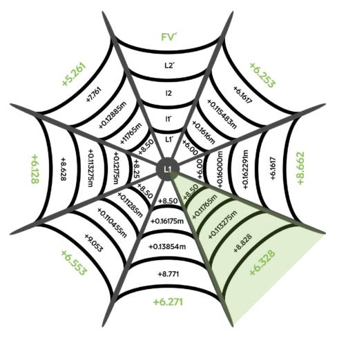
L1 = 0 L1' = L1 + F1 = 0 +8.50 = +8.50 = |1'=1/L1'=1/+8.50 = 0.11765m= |2=|1'-(t/n) = 0.11765m - (0.007/1.6) = 0.113275mL2 = 1/|2 = + 8.828L2'/FV' = L2 + F2 = +8.828 + -2.50
