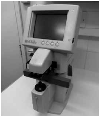
Figure 10.12a Electronic focimeter also known as projection focimeter
