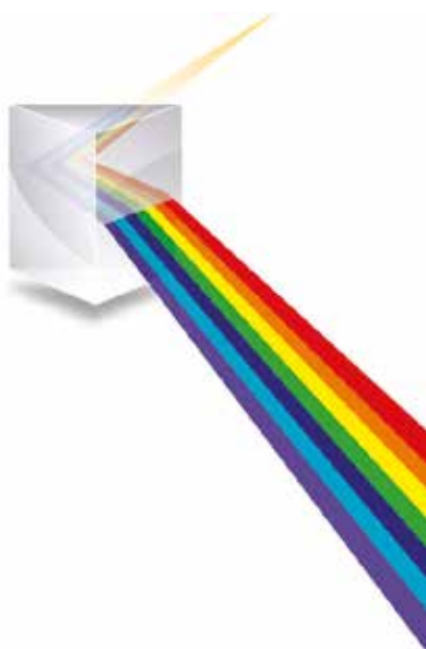
Figure 5.4 The refraction of the various coloured components of white light by a prism
