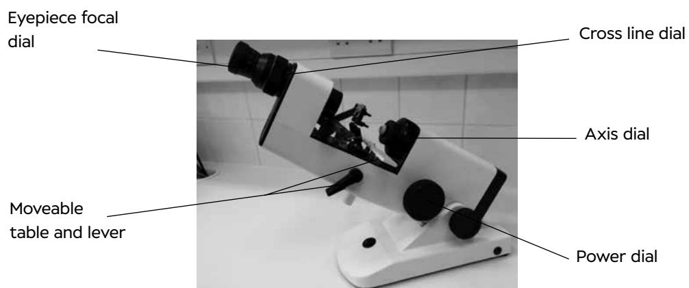
Figure 10.12b Labelled diagram of manual focimeter also known as target focimeter
