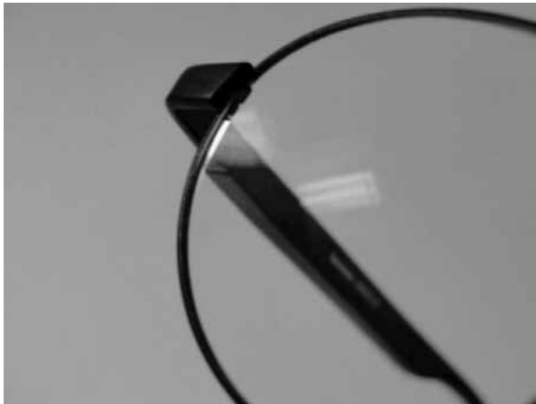
Figure 10.9. Notice how the UltraClear treatment does not go all the way to the edge of the lens
